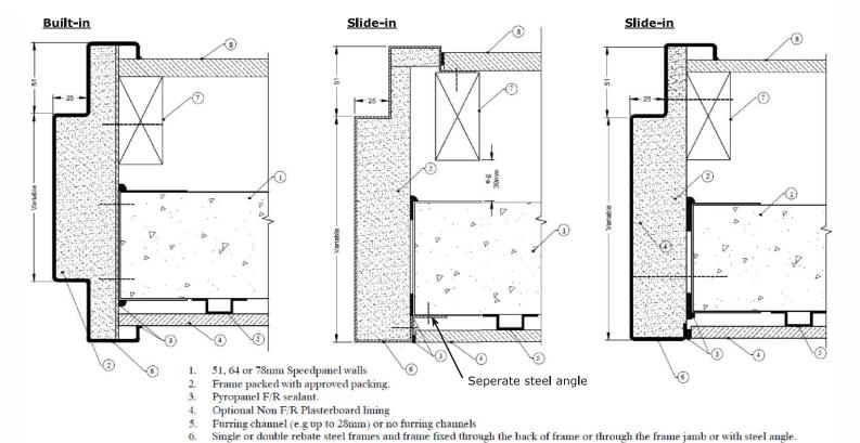
**Note:** Approved frame packing materials: Fire rated plasterboard, Pyropanel M4 lightweight mortar or mortar. Frames screw fixed at nominal 400mm centres.
