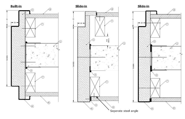
**Note:** Approved frame packing materials: Fire rated plasterboard, Pyropanel M4 lightweight mortar or mortar. Frames screw fixed at nominal 400mm centres.
