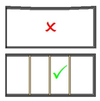
3. The transport spreaders at the base or the frame are not intended to be used during installation and must be removed. Spreaders need to be removed with a grinder, as twisting or knocking off will deform the frame. The frame must be installed with a timber or equivalent spacer cut to the same reveal width as the top of the frame, installed at the base and middle at a minimum. See below. Timber spacers must support the total width of the frame.
