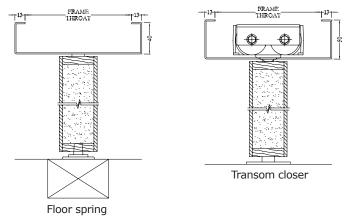
Typical head and floor section detail
